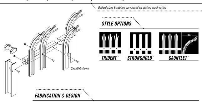
The Stalwart IS system is manufactured of high-tensile steel and is pre-galvanized inside and out for superior corrosion protection. Each component has been roll-formed into a unique profile that yields significant strength properties to encourage an anti-climb and anti-cut perimeter barrier. Each connection point of the Stalwart IS system is secured with tamper-proof fasteners providing the highest level of security and versatility.
