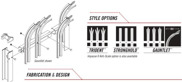
Impasse II panels and posts are manufactured using high-tensile pre-galvanized G-90 steel. Each component has been roll-formed into a unique profile that yields significant strength properties. Impasse II's distinct design enables the fence to traverse aggressive changes in grade in order to maintain security along any perimeter. Each connection point of the Impasse II system is secured with tamper-proof fasteners providing the highest level of security and versatility.
