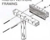
Note that kits for gate openings over 14' contain two track pieces. These are simply joined by stainless steel pins press fit into pre-machined alignment holes in the ends of the track extrusions.
