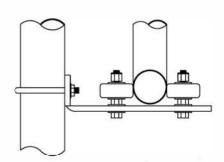
END VIEW OF INSTALLED LOWER GUIDE ROLLER ASSEMBLY (included with kit)
