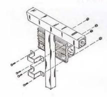
4. BOLTED DIRECTLY TO HORIZONTAL AND/OR VERTICAL FRAMING
